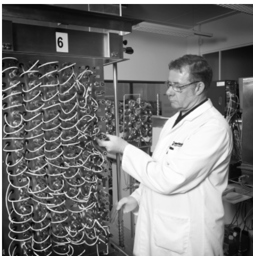
Calibrating dew-point transmitters in Michell's UKAS accredited calibration laboratory
