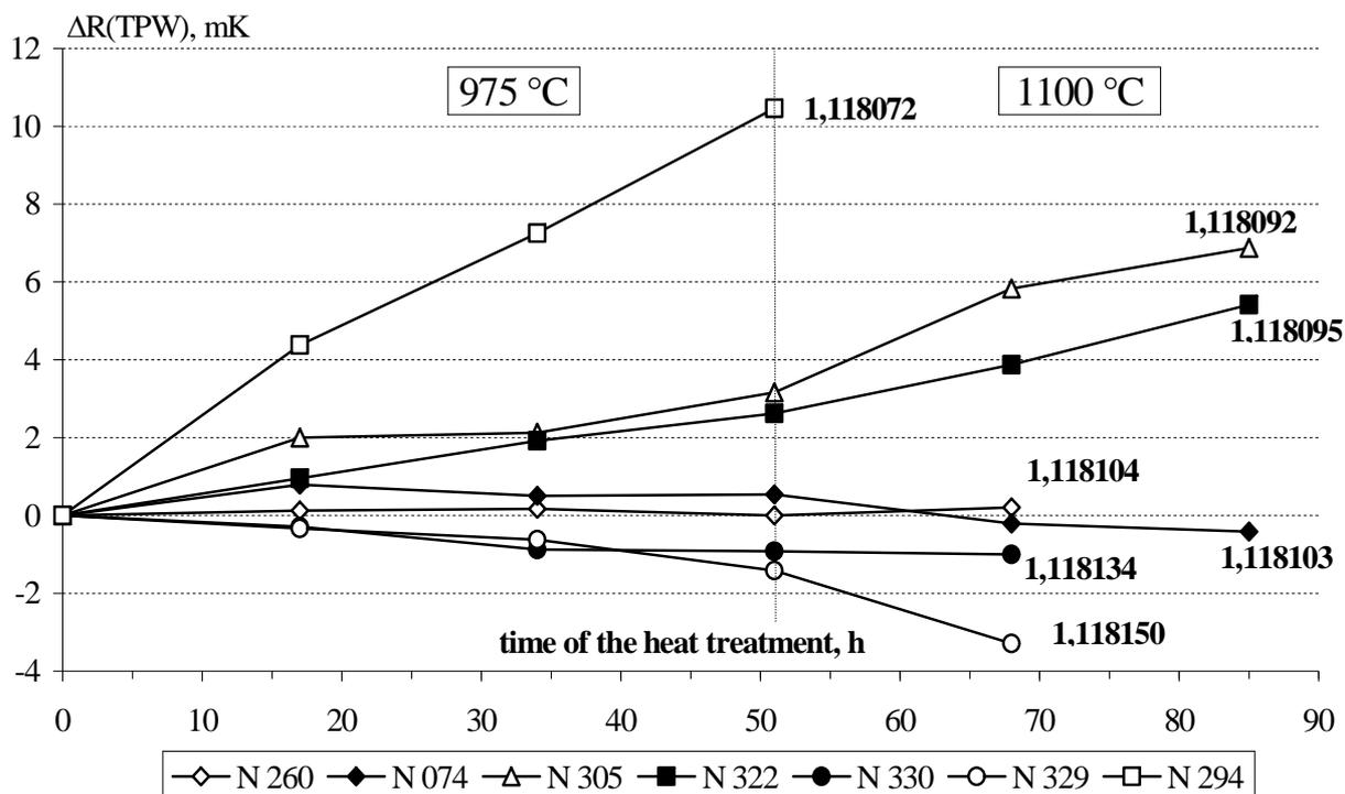
**Figure 5:** Change in  $R(TPW)$  during the simultaneous heat treatment of HTPRTs with different  $W(Ga)$  values.
