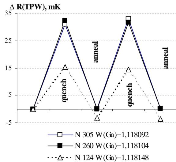
**Figure 4:** Change in R(TPW) during quench and anneal of HTPRTs
