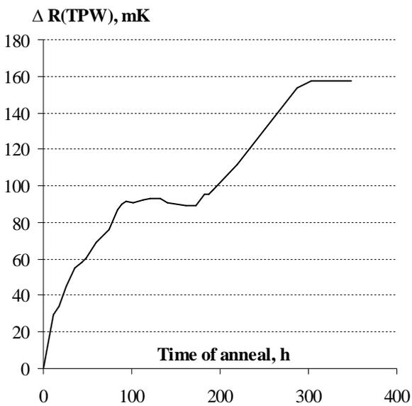
**Figure 3:** Change in R(TPW) during heat treatment of HTPRT N307, W(Ga)=1.118085
